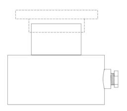
Media replacement is a simple procedure. The 2 inch threaded plug is removed and the spent media is dumped out. The new media is then installed, shaken down to reduce void space and the plug screwed back into place.
