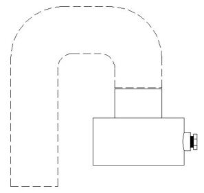
**VENT PURE-G** units are made from PVC for chemical resistance. The top is screened so inverted mounting is recommended if water will lie on top. Standard inlet pipe sizes for **VENT PURE-G** filters are 4, 6 and 8 inches. Other sizes are available upon request.
